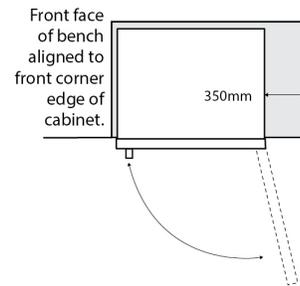
When positioned in a corner area, spacing of at least 400mm on the hinge side will allow the doors to open enough to enable the removal of bins and shelves.
