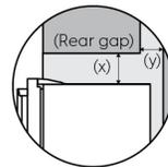
If gap (Y) is not minimum of 100mm, then gap (X) increases from 50 to 90mm min.
