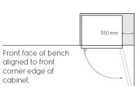
When positioned in a corner area, spacing of at least 350mm on the hinge side will allow the doors to open enough to enable the removal of bins and shelves.
