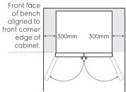
When positionec in a corner area, spacing of at least 300mm on the hinge side will allow the doors to open enough to enable the removal of bins and shelves.
