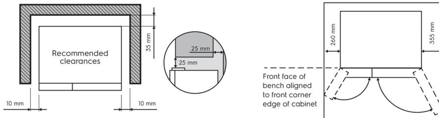
When positioned in a corner area, spacing of right side at least 260 mm and left side at least 355 mm on the hinge side will allow the doors to open enough to enable the removal of bins and shelves.
