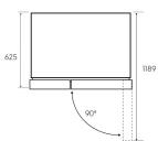
Front face of bench aligned to front corner edge of cabinet.
