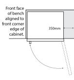
When positioned in a corner area, spacing of at least 400mm on the hinge side will allow the doors to open enough to enable the removal of bins and shelves.
