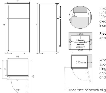
If you have a cupboard above the refrigerator with a rear gap of less than 100mm (Y), recommended minimum clearance at the top of the refigerator increases from 30mm to 70mm (X).
