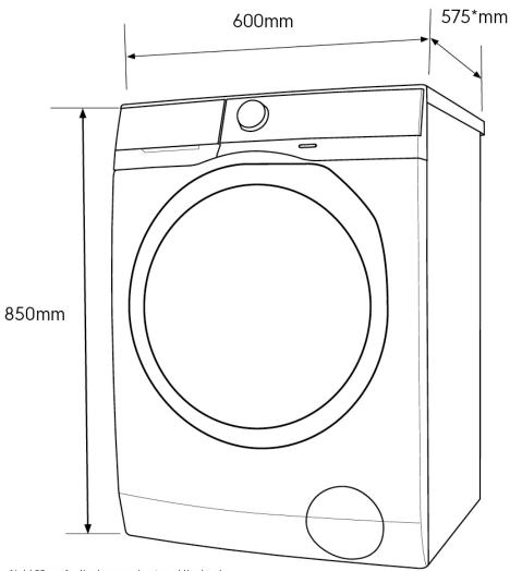
\*Add 20mm for the hose protrusion at the back.
