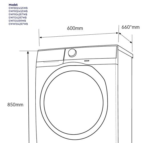
\*Add 20mm for the hose protrusion at the back.
