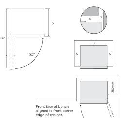
If you have a cupboard above the refrigerator with a rear gap of less than 100mm (Y), recommended minimum clearance at the top of the refrigerator increases from 30mm to 70mm (X).
