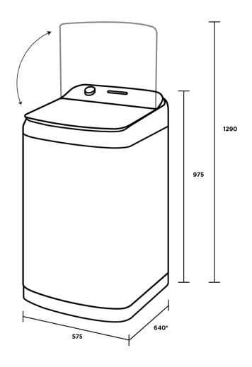
\*Add 25mm for the hose protrusion at the back
