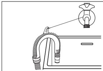
In this case, make sure the end cannot come unhooked when the machine will be emptied.
