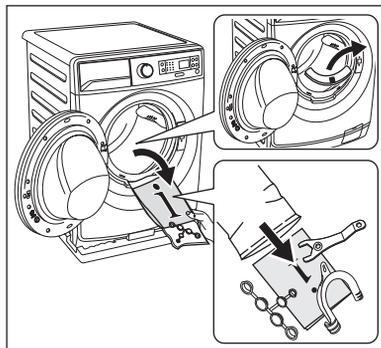
6. Put one of the polystyrene packaging elements on the floor behind the appliance. Carefully put down the appliance with the rear side on it. Make sure not to damage the hoses.
