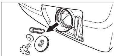
7. Make sure that the impeller of the pump can turn. If this does not occur, contact the service centre.
