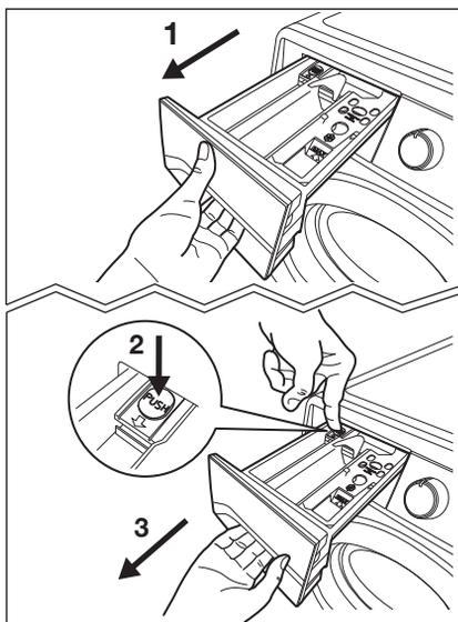
To aid cleaning, the top part of the additive compartment should be removed.
