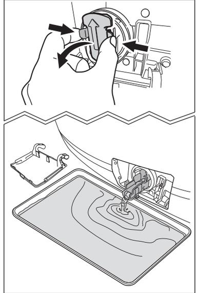
4. When the container is full of water, put the drainage duct back again and empty the container. Do step 3 again and again until no more water flows out from the drain pump.
