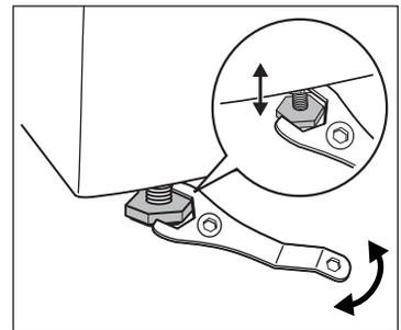
When the washer-dryer is levelled, try to rock it from corner to corner. If it does rock, adjust the legs again until it is levelled and does not rock.
