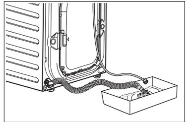
5. When no more water flows, install the inlet hose and the drain hose again.
