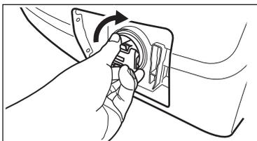
10. Put the flap back and close the drain pump door.
