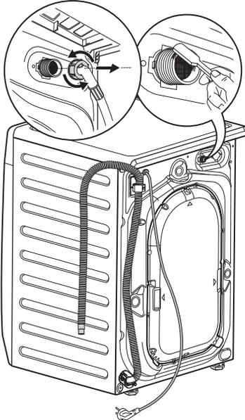
6. Install the inlet hose again. Make sure that the couplings are tight to prevent leakages.
