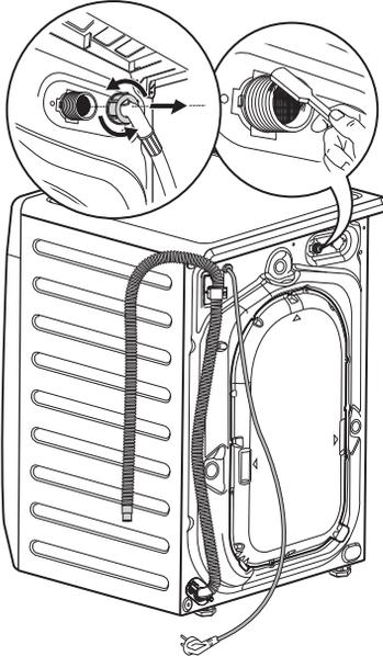
6. Install the inlet hose again. Make sure that the couplings are tight to prevent leaks.
