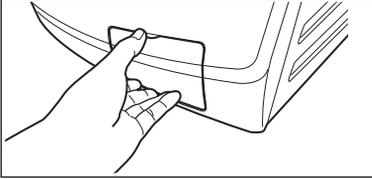
2. Pull the flap down, then squeeze the legs on both sides of the cover together and pull out (as picture).
