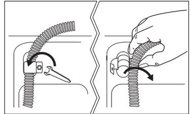
4. Put the end of the drain and inlet hose in a container. Let the water flow out of the hoses.
