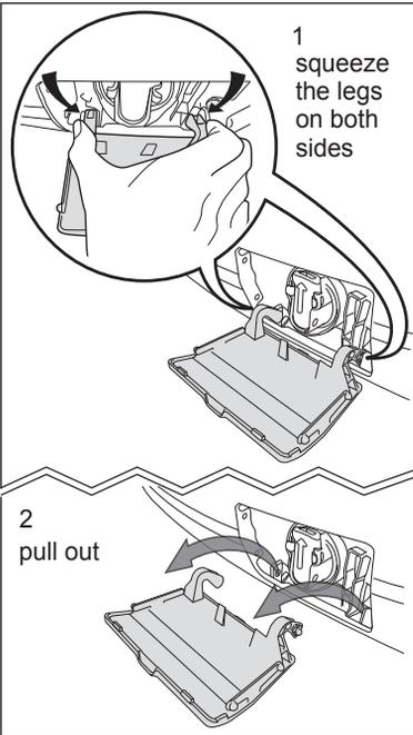
3. Place a suitable water container below the recess of the drain pump to collect the water that flows out. Press the two levers and pull forward the drainage duct to let the water flow out.
