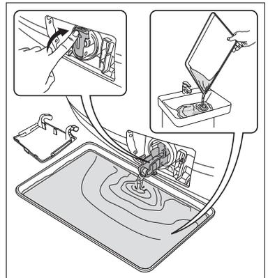
5. Pull back the drainage duct and turn the filter counter-clockwise to remove it.
