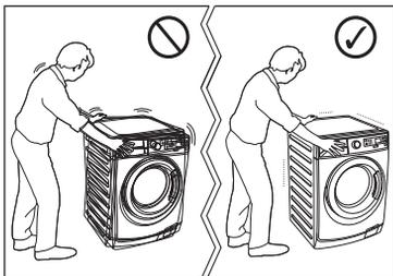
Never place cardboard, wood or similar materials under the machine to compensate for any unevenness in the floor. Install the machine on a flat hard floor. Make sure that air circulation around the machine is not impeded by carpets, rugs etc. Check that the machine does not touch the wall or cupboard units.
