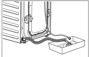
5. When no more water flows, install the inlet hose and the drain hose again.
