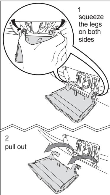
3. Place a suitable water container below the recess of the drain pump to collect the water that flows out. Press the two levers and pull forward the drainage duct to let the water flow out. Press the two levers and pull forward the drainage duct to let the water flow out.
