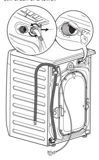
Install the inlet hose again. Make sure that the couplings are tight to prevent leakages.
