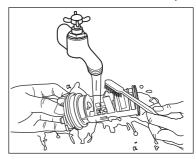
Put the filter back in the pump into the special guides. Make sure that you correctly tighten the filter to prevent leakages.
