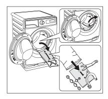
Put one of the polystyrene packaging elements on the floor behind the appliance. Carefully put down the appliance with the rear side on it. Make sure not to damage the hoses.
