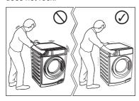
Never place cardboard, wood or similar materials under the machine to compensate for any unevenness in the floor. Install the machine on a flat hard floor. Make sure that air circulation around the machine is not impeded by carpets, rugs etc.
