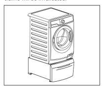
To put the appliance higher at the level what helps easy load and remove the laundry.
