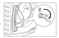
To disable this device and restore the possibility of closing the door, rotate the button counter-clockwise until the groove is vertical.
