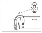
In this case, make sure the end cannot come unhooked when the machine is emptying.
