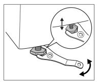
When the washing machine is levelled, try to rock it from corner to corner. If it does rock, adjust the legs again until it is levelled and does not rock.
