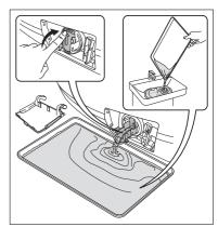
Pull back the drainage duct and turn the filter counter-clockwise to remove it
