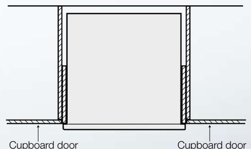
For the best integration within a kitchen, install this appliance in a standard 600mm wide cupboard that gives a flush fit with the surrounding cupboard fronts (Figure 1). A 20mm recess is ideal. It can also be installed using a proud fit with the surrounding cupboard (Figure 2).
