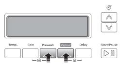
By pressing the "Prewash" and "Vapour" buttons simultaneously for about 6 seconds, the acoustic signal is deactivated (except for the events of operating problems).
