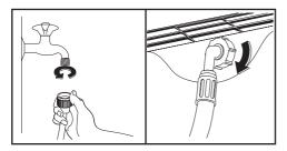
The inlet hose must not be lengthened. If it is too short and you do not wish to move the tap, you will have to purchase a new, longer hose specially designed for this type of use.
