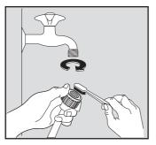
Turn off the water tap. Unscrew the water inlet hose. Clean the filter using a hard bristle brush. Tighten up the inlet hose.
