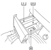
Always add laundry detergents before switching the machine on and keep the dispenser clean and dry, so that the detergent can be efficiently dispensed from the unit.
