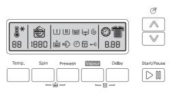
Depending on the program, different functions can be combined. These must be selected after choosing the desired program and before depressing the **Start/Pause** button.
