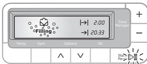
To start the selected programme, press the “**Start/Pause**” button; the corresponding green pilot light stops flashing.
