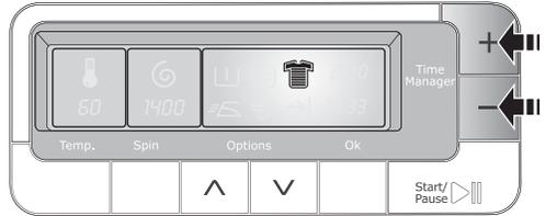
This function allows you to modify the washing time, automatically proposed by the washing machine.
