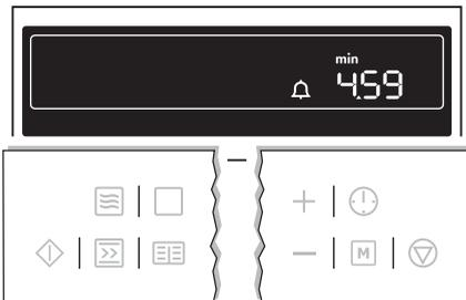
When the time set has elapsed, an acoustic signal sounds for 2 minutes. "0.00" lights up and the symbol for Countdown
