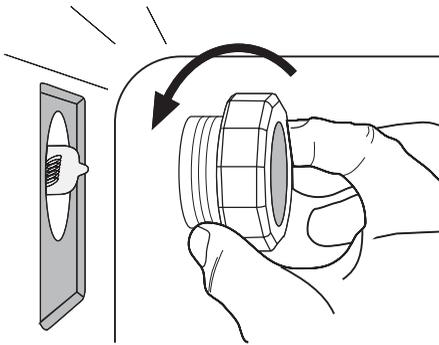
3. If necessary: Replace with halogen oven light bulb 20 Watt, 12 V, 300°C heat-resistant.
