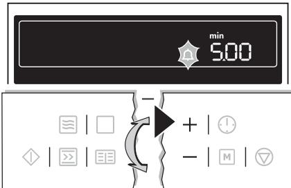
After about 5 seconds the display shows the time remaining. The symbol for Countdown
