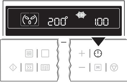
3. Using the End time
