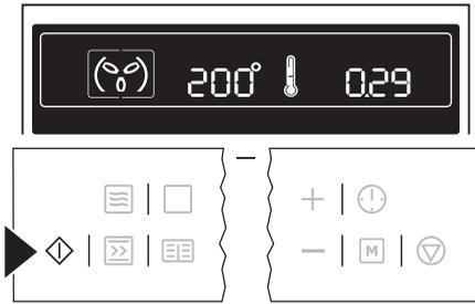
2. Press the Clock Functions  $\text{⌚}$  button repeatedly until the symbol for End time  $\rightarrow$  flashes.
