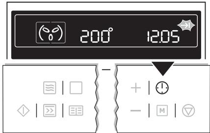
3. Using the + or - button, set the desired switch-off time.
