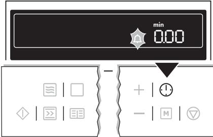
2. Using the + or - buttons, set the desired countdown (max. 99.00 minutes).
