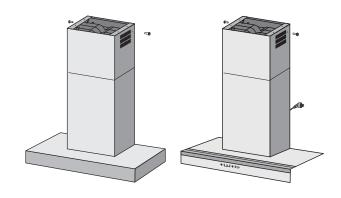
Insert carbon filter into position and replace the grease filters over fan inlet.
