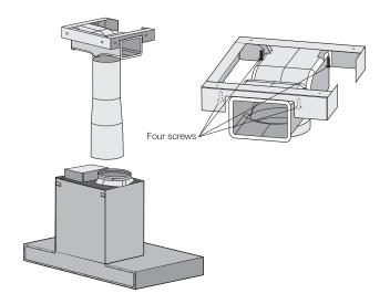
**step 4:** Carefully lower the assembled inner and outer exhaust covers onto the top of the cooker hood body, and insert the exhaust cover into the rangehood body approximately 5mm. Fix inner (top) exhaust cover to the ceiling mounting bracket with screws supplied. Ensure that the inner (top) section is extended.
