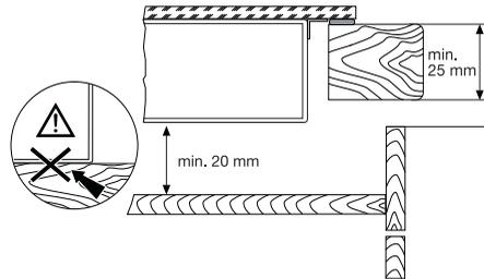
**Warning!** Surface temperatures of base exceed 95°C, under bench access must be restricted by use of non-combustible barrier on installation
