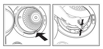
To remove the lint filter open the door and press the two pads together. Pull the lint filter out of the pocket.
