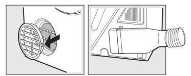
Inlet and outlet points need clear airflow to prevent overheating, so ensure there is adequate ventilation. (i.e. open window or external door.)
