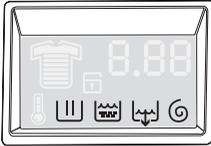
After the machine has started, only the running icon stays on. When the programme has finished, a flashing zero (0.00) is displayed.
