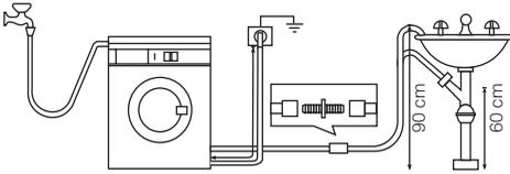
**For the correct functioning of the machine the drain hose must remain hooked on the proper support piece situated on the top part of back side of the appliance.**
