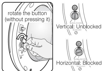
To disable this device and restore the possibility of closing the door, rotate the button anti-clockwise until the groove is vertical.
