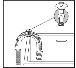
This could be done by tying it to the tap with a piece of string or attaching it to the wall.
