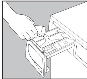
If required, pour fabric softener into the compartment marked
