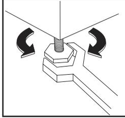
Never place cardboard, wood or similar materials under the machine to compensate for any unevenness in the floor.
