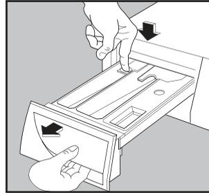
To aid cleaning, the top part of the additive compartment should be removed.
