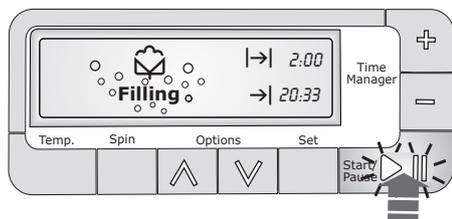
To start the selected programme, press the **“Start/Pause”** button; the green pilot light stops flashing.
