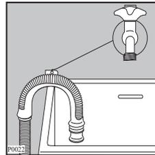
**In a sink drain pipe branch.** This branch must be above the trap so that the bend is at least 60 cm above the ground.
