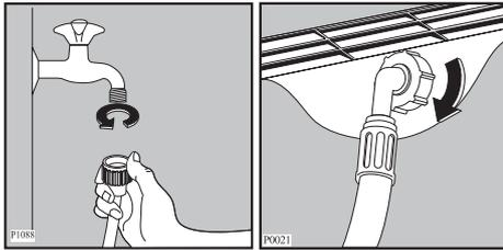
The inlet hose must not be lengthened. If it is too short and you do not wish to move the tap, you will have to purchase a new, longer hose specially designed for this type of use.
