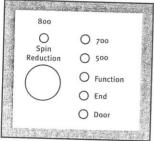
Function: when this light comes on this means that the machine is performing the washing programme.
