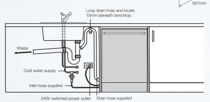
**Note:** Hole at bottom of spigot on sink drain must be drilled out completely. Position of spignot from base of dishwasher floor must be 300mm minimum. Maximum height of drain hose from floor must be 1000mm.
