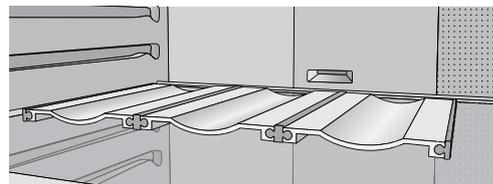
The Modular bottle caddy is made of anodised aluminium. They are used to store various types of bottles like wine or beer. Bottles should be stored with the bottom end towards the back of the refrigerator. The fridge arrives with three combined caddies, but they can be separated if desired.
