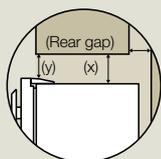
If you do not have a cupboard with a rear gap, the recommended clearance area on top increases from 50mm to 90mm (x) and from 32mm to 72mm (y).
