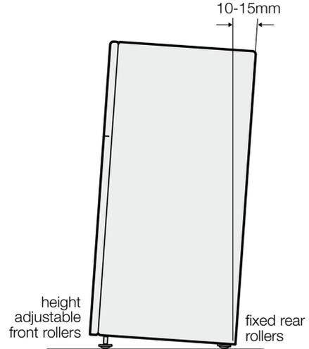
The stability foot should also be wound fully up so it will not interfere with the operation of the rollers (see diagram in Step 3).
