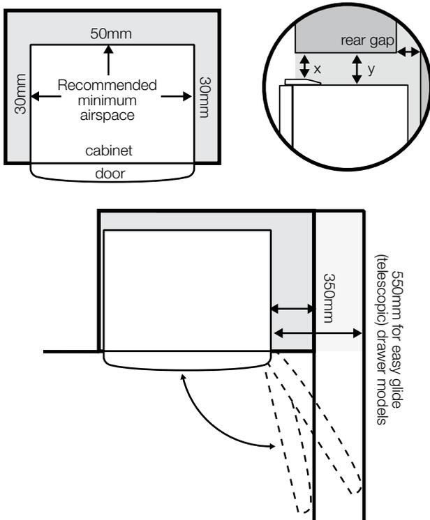
*NOTE: Doors are designed to sit proud of cabinetry (not flush). The clearances shown above are the recommended minimum clearances. The clearance at the rear must not exceed 75mm.*
