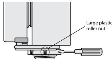
4. Check the alignment of the refrigerator to the surrounding cupboards to see if it is level. You can adjust the level with the rollers as detailed in step 3.
