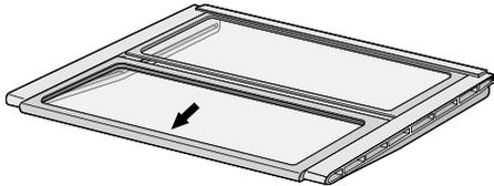
2. Then, from the underside, lift the front half of the shelf by raising the rear edge over the recessed hook detail.
