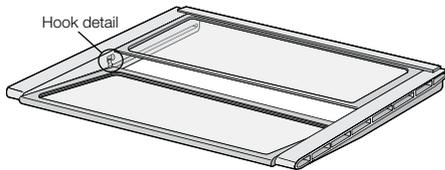
3. Pull the shelf forward and allow the rear to drop into the side channels.
