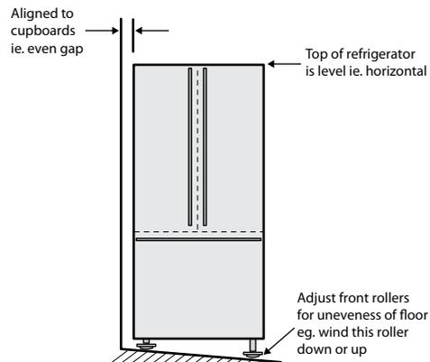
5. After you have tried Step 3 and 4, and still find your refrigerator rocks from corner to corner, it means your floor is uneven. Find a piece of plastic or hardboard etc. and pack it firmly under the rear roller.
