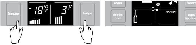
Press and hold the freezer and fridge buttons together to activate the child lock. This will disable the display to prevent accidental changes to settings. To turn the child lock off, press and hold the freezer and fridge buttons together.
