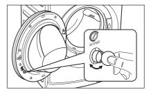
To disable this device and restore the possibility of closing the door, rotate the button anti-clockwise until the groove is vertical.
