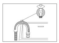
In this case, make sure the end cannot come unhooked when the machine is emptying.
