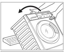
6. Put one of the polystyrene packaging elements on the floor behind the appliance. Carefully put down the appliance with the rear side on it. Make sure not to damage the hoses.
