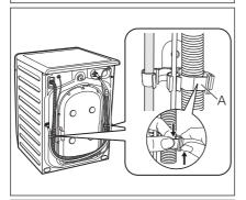
9. Remove the power supply cable and the drain and inlet hoses from the hose holders (A) on the rear of the appliance.
