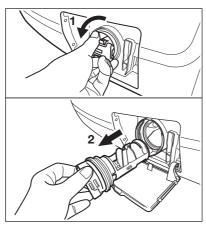
6. Pull back the drainage duct and turn the filter to remove it.
