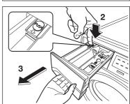
To aid cleaning, the top part of the additive compartment should be removed.
