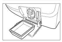
Put a container below the recess of the drain pump to collect the water that flows out.
