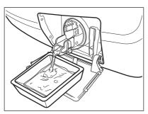
When the container is full of water, put the drainage duct back again and empty the container. Do steps 4 and 5 again and again until no more water flows out from the drain pump.
