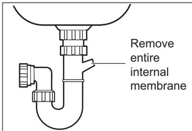
If you connect the water drain hose to a trap spigot under the sink, remove the plastic membrane. If you do not remove the membrane, remaining food can cause a blockage in the drain hose spigot.
