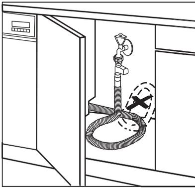
In order to pass the safety valve through the kitchen cabinets, an opening of at least 45 mm x 90 mm is needed.
