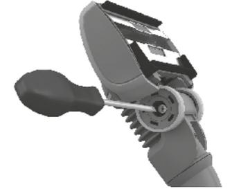
Unscrew the wheel axis and clean all parts. Refit in reverse order.
