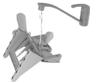
7. Open the fine dust container lid and wash the dust container with water. Wash the fine dust container every 2 years.
