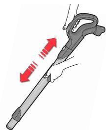
4. **Adjust the telescopic tube** by holding the lock with one hand and pulling the handle with the other hand.
