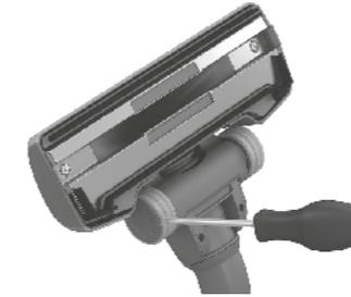
If the wheels are stuck, clean them by removing the wheel cap with a small screwdriver.
