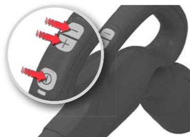
9. **Press the On/Off button to turn on and off.** Press '+' to increase power and press '-' to reduce power.\*
