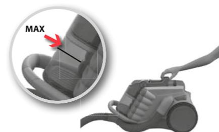
1. **Dust compacting:** When max level is reached, compact dust gently.
