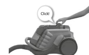
3. **Pull compactor handle back and continue cleaning until compacted dust reaches max level. Hear the click to ensure the dust compactor is locked in properly.**
