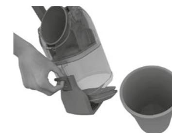
2. **Unlock button and push downwards to release bottom lid.**
