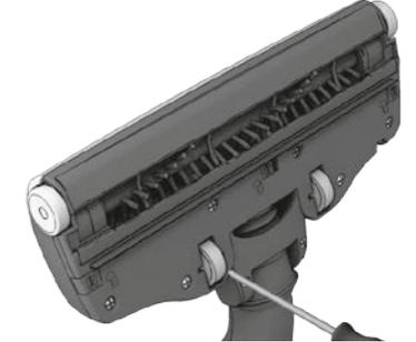
If the wheels are stuck, remove them carefully by using a small screwdriver.
