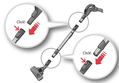
3. **Attach the telescopic tube to the floor nozzle and hose handle** (to remove them, press the lock button and pull the nozzle and hose off).
