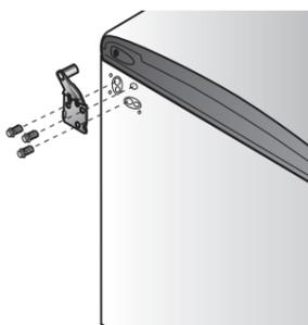
7. Remove freezer door by opening 45° and gently slide off hinge. Set door aside to prevent damage.
