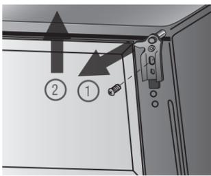
15. Place the base support RH (kit contents) onto the cabinet, placing it down then towards cabinet to install. Replace the screw.
