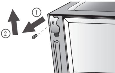
17. Place the bottom hinge LH (kit contents) onto the cabinet, placing it down then towards cabinet to install. Replace the screw.
