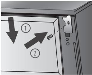
16. Unscrew the base support LH screw shown, pull the support away from cabinet then up to remove.
