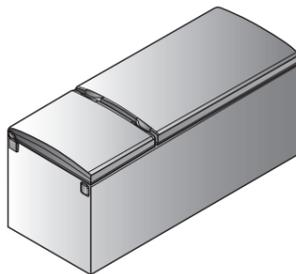
4. Remove the hinge cover with a soft plastic lever.
