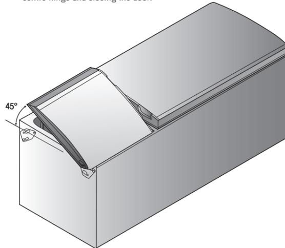
23. Slide the LH top hinge (kit contents) into the door, loosely screw the 3 x 8mm screws from the existing top hinge in the cabinet.
