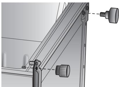
19. Replace the food door by holding at 45° and gently slide onto the bottom hinge and closing the door.
