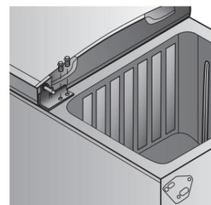
9. Remove RH centre hinge by lifting the door slightly and sliding hinge out of the door.
