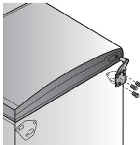
24. Ensure that the edges of the doors are parallel with the sides of the cabinet.
