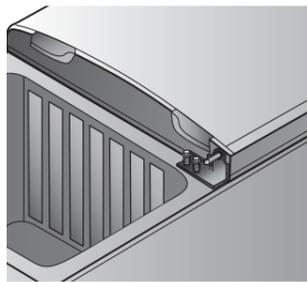
22. Replace the freezer door by holding at 45° and gently slide onto the centre hinge and closing the door.
