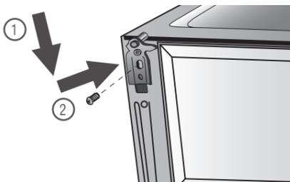
18. Replace the hinge foot onto the LH bottom hinge and tighten with screw. Screw the other foot into the corresponding hole.
