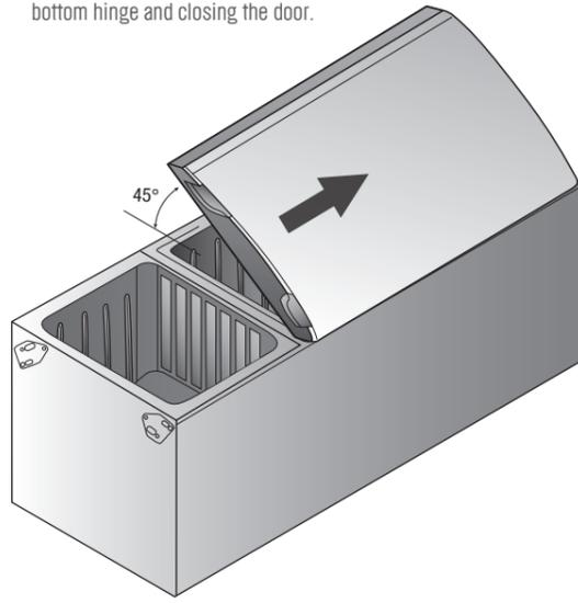
20. Replace LH centre hinge by lifting the door slightly and sliding hinge into the door and placing the door down again.
