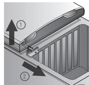
10. Remove food door by opening 45° and gently slide off hinge. Set door aside to prevent damage.
