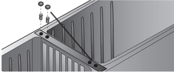
13. Unscrew the hinge foot using phillips head screwdriver and unscrew foot on opposite side. Do not discard.
