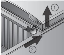
21. Insert 2 x 8mm screws from existing centre hinge into the LH centre hinge, tighten the screws until the bracket is secured.
