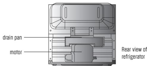
3. Lay the refrigerator on its back.
