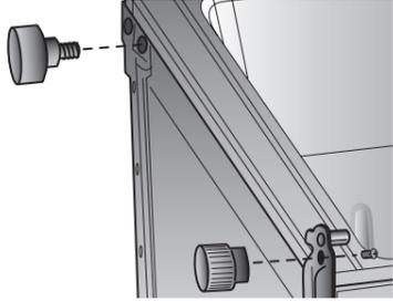
14. Unscrew the bottom hinge screw shown, pull the hinge away from cabinet then up to remove.
