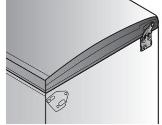
27. Clip the LH hinge cover (kit contents) over LH top hinge.
