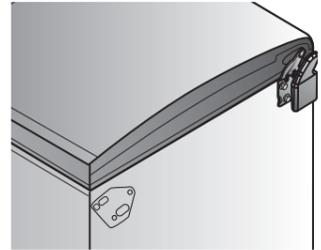
28. Insert the RH top hinge hole cap (kit contents) in the cabinet as shown.
