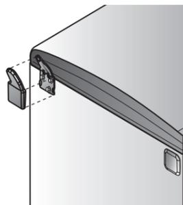
5. Remove the LH cap with a soft plastic lever.
