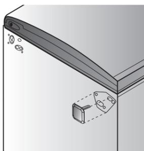
6. Unscrew 3 x 8mm top hinge screws and remove RH top hinge. Do not discard screws.
