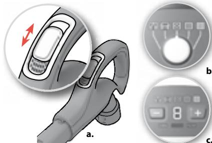
**9. Adjust suction power.** Models with manual regulation. a) Use the suction control on the handle to quickly reduce the airflow b) Use the rotary knob on the cleaner to adjust suction power c) Use the + or - button on the cleaner to adjust suction power.\*
