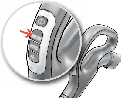
**11. Models with remote control and Aeropro motorized nozzle.** To turn the motorized nozzle on and off, press BRUSH button on the handle.\*
