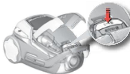
Press the 3in1 button to open the compartment. After usage, put the accessory back in its place.
