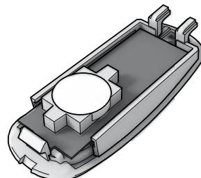
**2. Use only batteries type LITHIUM CR2032.** Batteries must be removed from the appliance before it is scrapped and are to be disposed of safely.
