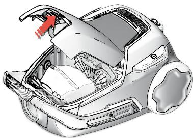
1. Open the dust compartment cover by pulling the s-bag button. **Check that the s-bag® is in place.**
