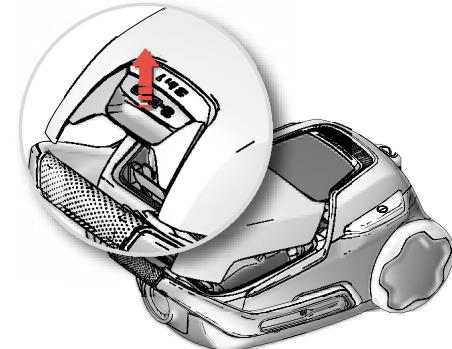
3. Open the dust compartment cover by pulling the S-BAG button.
