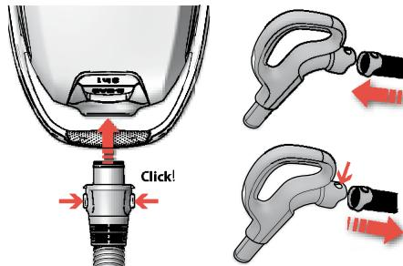
2. Insert the hose into the cleaner (to remove it, press the lock buttons and pull the hose out).
