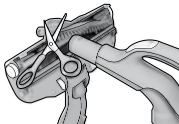
2. Pull out the brush roll and remove entangled threads by snipping them away with scissors. Use the hose handle to clean the nozzle. Refit in reverse order.
