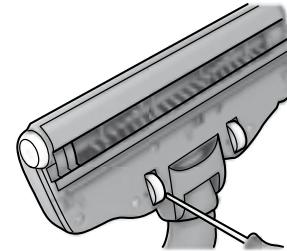
3. If the wheels are stuck, remove them carefully by using a small screwdriver and clean the wheels.
