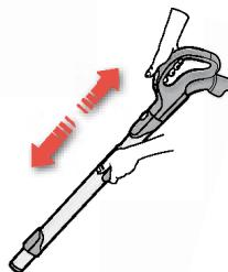
5. Adjust the telescopic tube by holding the lock with one hand and pulling the handle with the other hand.
