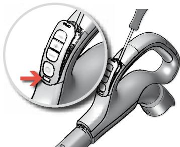
**1. Models with remote control:** Change battery when light indicator on handle turns red or is not responding when pressing any button.\*
