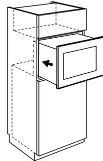
5. Open the door and fix the appliance to the cabinet with a screw.
