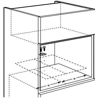
4. Install the appliance. Make sure the bracket locks the back of the appliance.
