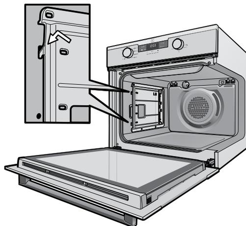
1. Position the first liner as per the diagram. The black, shiny side of the liner should be facing the oven wall with the hooks pointing down. Note that the diagram shows the left hand liner. The right hand side will be a mirror image of this.
