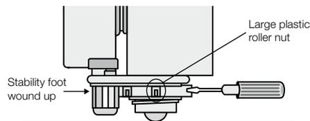
4. Check the alignment of the refrigerator to the surrounding cupboards to see if it is level. You can adjust the level with the rollers as detailed in step 3.
