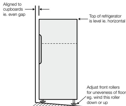
5. If you find your refrigerator rocks from corner to corner, it means your floor is uneven. Find a piece of plastic or hardboard etc. and pack it firmly under the roller.
