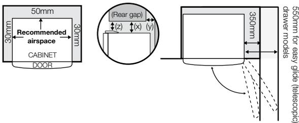
**NOTE:** Doors are designed to sit proud of cabinetry (not flush). The clearances shown above are the recommended minimum clearances. The clearance at the rear must not exceed 75mm.
