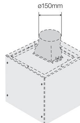
*NOTE: The fan housing flue transition duct is 150mm in diameter. (See page 10 for optional ducting accessories).*
