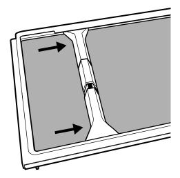
6. Release the latch handle when the Bottle Lock is in the desired position in order to lock the latch to the crisper shelf.
