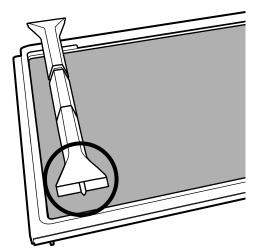
2. Insert the latch end under the lip at the front of the crisper shelf at either side.
