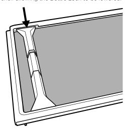
4. Slide the latch handle back to retract the latch.
