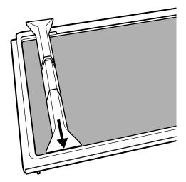
3. Lower the back of the bottle lock onto the crisper shelf. There is a gap in the back lip of the crisper shelf allowing the Bottle Lock to be lowered.
