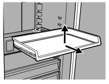
3. Pushing the tab gently inwards on both sides of the frame, pull the frame towards you to remove it from the cabinet.
