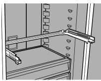
2. Push the frame straight inwards until its clip gets locked in the rear pocket.
