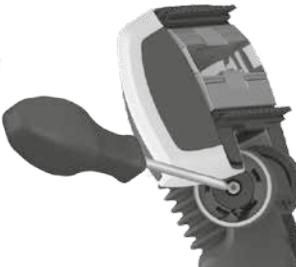
3. Unscrew the wheel axis and clean all parts. Refit in reverse order.
