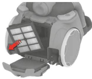
2. Remove the HEPA filter and rinse with cold water.
