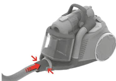
2. **Insert the hose into the connection at the front** (to remove it, press the lock buttons and pull the hose out).
