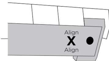
5. Once both crispers are installed, check to ensure the crisper cover is fixed into place, and that clearances between the crisper and the crisper cover are even
