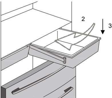
4. Ensure that the crisper is fully engaged with the rubber block and aligned as shown in the image.
