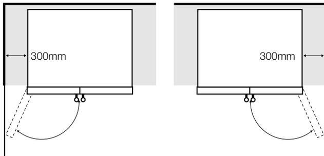
*NOTE: Doors are designed to sit proud of cabinetry (not flush). The clearances shown above are the recommended minimum clearances. The clearance at the rear must not exceed 75mm.*
