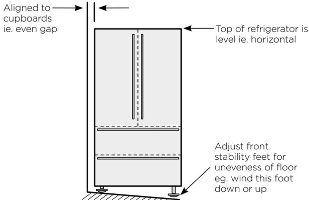
5. If you find your refrigerator rocks from corner to corner, it means your floor is uneven. Find a piece of plastic or hardboard etc. and pack it firmly under the foot.
