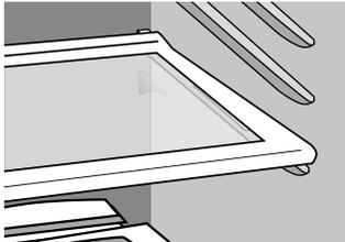
Spillsafe™ glass shelves keep spills on the shelf. A shelf retaining system minimises accidental movement of shelves and they can be adjusted to various heights. Spillsafe™ glass shelves are not to be used as slide out shelves. To remove the shelves, gently pull them forward until the shelf comes out.
