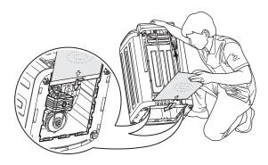
**3.** Lie down the washing machine on its back, taking care not to damage cabinet by placing
