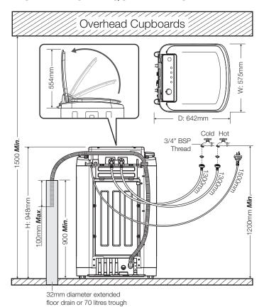
1. Electrical: A properly earthed three pin power point not more than 1500 mm from the washing machine. It is not recommended that an extension cord be used. If you need to use an extension cord or portable outlet, make sure that it is not subject to splashing or ingress of moisture.
