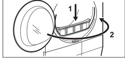
1) If necessary clean the filter with tap warm water using a brush and/or a vacuum cleaner.
