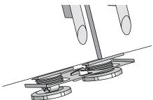
7. With the two cabinets provisionally connected, level both units using adjustable rollers as per recommendations in your owner's manual. Gently push the assembly back into the wall cavity and check for alignment and level. If necessary, pull the cabinets out again and adjust, repeat the procedure until satisfied with level and alignment.
