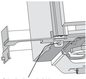
Tension on the centre cover can be adjusted with the screw on the bottom bracket
