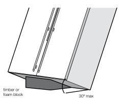
Tilt the cabinet back by no more then 30 degrees. This will enable adequate access to the front feet in order to install lower bracket. Ensure that assistant has firm grip of the cabinets before continuing. Use chocks or other means of firmly supporting the cabinets before attempting further installation work. The cabinets can be best tilted by having assistant pull and support the appliances from the back.
