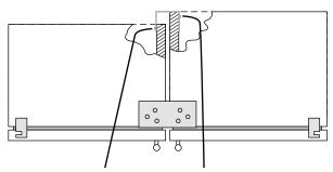
Two cabinets of different depths joined at the back with rear clamp. Notice that compressor mounting plate fasteners are in a different location on the rear clamp.
