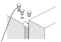
Carefully remove hole plugs from holes to allow fitment of the top bracket.
