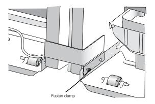
9. Adjust tension on centre cover for flush mounting with cabinets.
