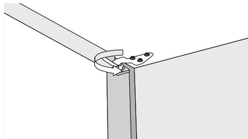
Loosening the top hinge fasteners will allow the top hinge to be slightly rotated thus adjusting the gap between doors.
