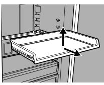
Pushing the tab gently inwards on both sides of the frame, pull the frame towards you to remove it from the cabinet.
