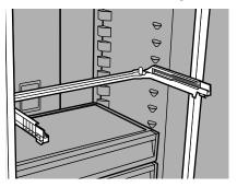
Push the frame straight inwards until its clip gets locked in the rear pocket.
