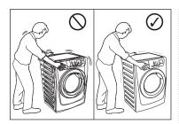
Never place cardboard, wood or similar materials under the machine to compensate for any unevenness in the floor.
