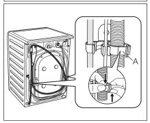
Remove the power supply cable and the drain and inlet hoses from the hose holders (A) on the rear of the appliance.
