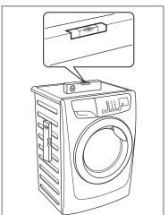
If you do not have a spirit level, as a guide use the edge of a door frame, cupboard or bench to check that the washing machine is level.
