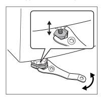
When the washing machine is levelled, try to rock it from corner to corner. If it does rock, adjust the legs again until it is levelled and does not rock.
