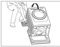
Put one of the polystyrene packaging elements on the floor behind the appliance. Carefully put down the appliance with the rear side on it. Make sure not to damage the hoses.
