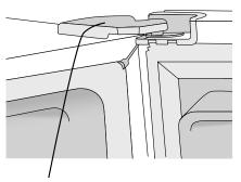
Small plastic clip is located here. With the door open, pull the cover outward while simultaneously pulling up in order to release the hinge cover.
