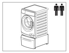
**12.** For tumble dryer. Unscrew and retain the two bottom screws from the back of the appliance.
