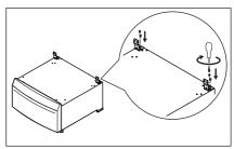
**14.** For tumble dryer. Lift the appliance and slide backwards so that the appliance front feet slides under foot locking brackets.
