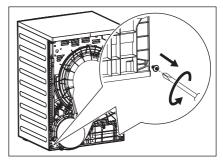
**13.** For tumble dryer. Screw the rear brackets (C) on the pedestal by using the screws supplied in the stand box.
