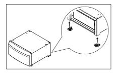
**3.** Adjust the front adjustable feet to make the pedestal stable.
