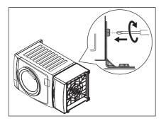
**11.** For washing machine. Put the pedestal and appliance in vertical position. If necessary, adjust the appliance feet and go to step 16. Check that the screws are firmly screwed.
