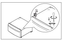
For washing machine. Gently lay the washing machine on its detergent dispenser side.
