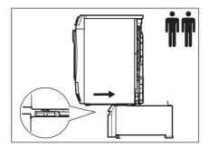
**15.** For tumble dryer. Screw the rear brackets (C) to the back of the appliance by using the screws removed in step 12 and adjust the appliance feet if required.
