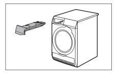
6. Screw the front brackets on the pedestal.
