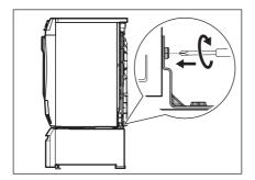
16. Move the Pedestal/Appliance assembly to its permanent location. Use a spirit level to check if the assembly is properly leveled. If not leveled, adjust feet to level properly.
