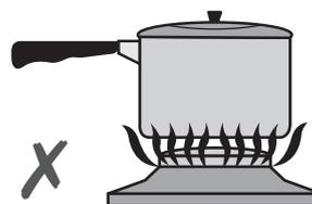
Incorrect – flame too high and will cause gas waste and possible handle damage.
